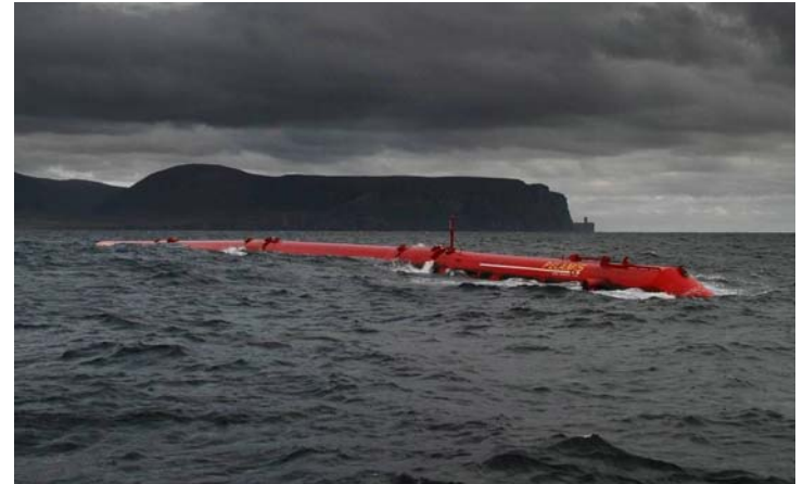
Pelamis wave energy system in testing
