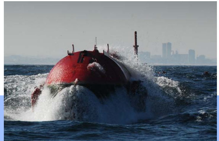
Pelamis wave energy system in testing
