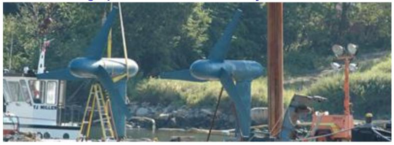
Initiated in 2002, the RITE Project demonstrates and delivers commercial electricity from Verdant Power's *Free Flow* Kinetic Tidal Hydropower System. Based on the success of the initial 6 turbines, work is currently progressing to add an additional 30, raising output to 1 megawatt.
