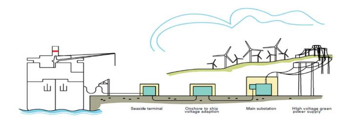
Shore connection is the electrical connection between the ship docked at the port and the dockside, in order to reduce both carbon emissions and acoustic pollution. It is obtained by switching off power generators on board and using the power generated onshore
