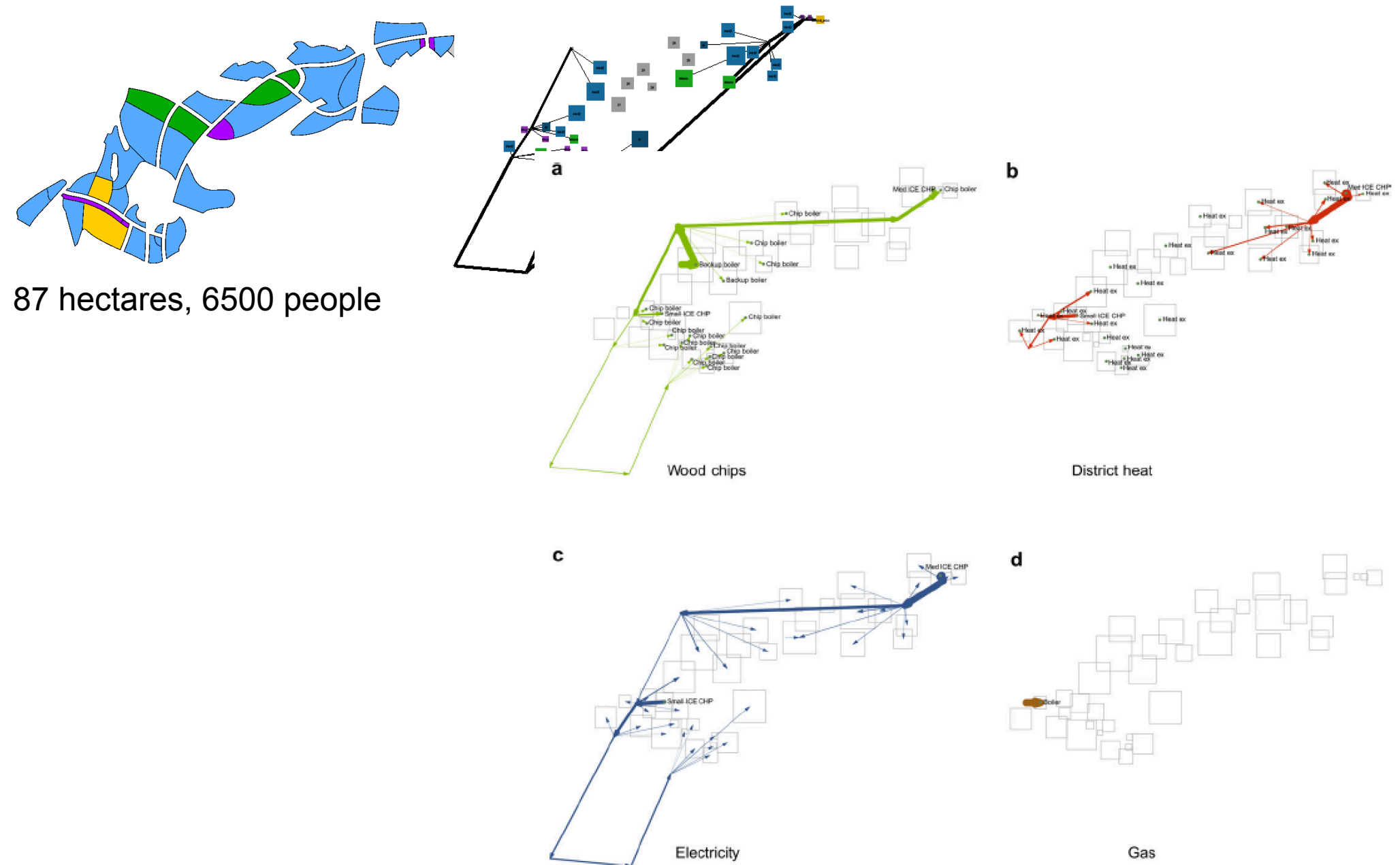
Fig. 3 – Distribution networks for the winter period of the all-technologies scenario (5). Arrow widths are proportional to resource flows.
